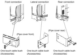
Note: Please ensure that the power cable and interconnecting cables are not installed through the same cable bush hole opening. They must be installed into the two separate hole openings to prevent damage to the cable.
