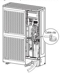
(4) Be sure to install the insulation sheet after the wiring is complete.
