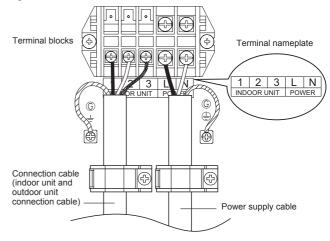
Secure the cables using the cable clips under the terminal blocks, and then secure the cables using the cable clips attached to the base of the valves.
