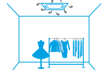
Air distribution with a dusty filter
