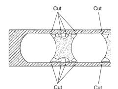
(3) Cut with nippers and remove the sheet metal
