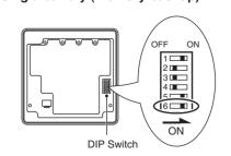
Change the DIP switch setting to use batteries. (The DIP switch If batteries are not used, all of the settings stored in memory will
