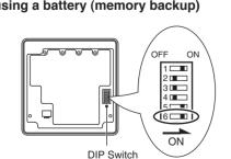
is not set to use batteries at the factory.) Change DIP switch No. 6 from OFF to ON.
