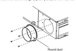
(3) Connect the duct to the round flange.
