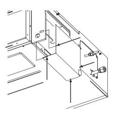
Adjust the position of the screws for control box cover according to the installation.
