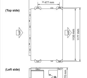
The distance of X is adjustable according to the place of the hanging bolts. (MAX: 550 mm, MIN: 410 mm)
