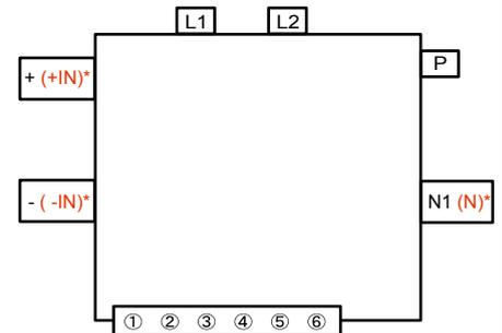
Check Point 2 : Check the Output DC voltage (between P and N)
