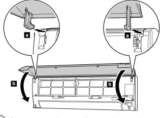
Press 4 places on the intake grille to close it completely. (4)
