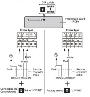
\*Earth (Ground) the remote controller if it has a earth (ground) wire.
