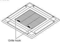
(2) Open the intake grille and remove.
