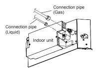
(3) When the flare nut is tightened properly by your hand, hold the body side coupling with a wrench, then tighten with a torque wrench. (Refer to the following table for the flare nut tightening torques.)
