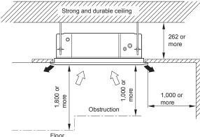
· This product can be installed at a height of up to 3,000mm. However, 7000, 9000 Btu/h model can not be installed in high places Perform the Function Setting on the remote control in accordance with the installed height. (Refer to "7. FUNCTION SETTING")
