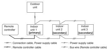
(2) Set the R.C. address (DIP switch setting) Set the R.C. address of each indoor unit using the DIP switches on the indoor unit circuit board. (Refer to the following table and figure.) The DIP switches are normally set to make the R.C. address "00"
