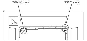
• Align the stamped marks on the cassette grille to the pipe and the drain of the indoor unit.
