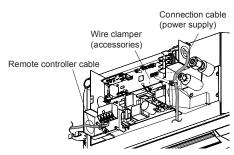
Do not bind the connection cable (power supply) and other cables together.
