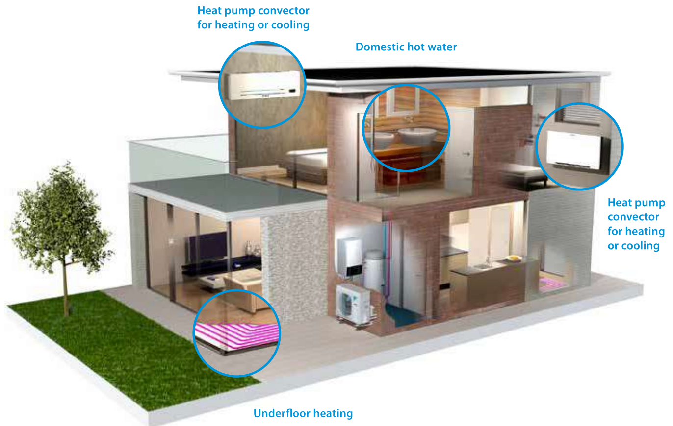
Example of installation with a stainless steel domestic hot water tank (EKHWS-D).
