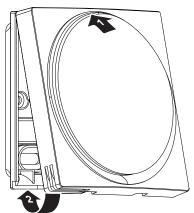
2 When the installation site is dust-free, peel off the protective
