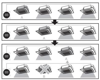
A Inactive backup unitB Unit in error
