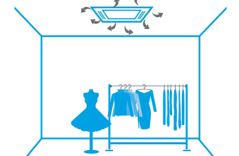
Air distribution with a dusty filter
