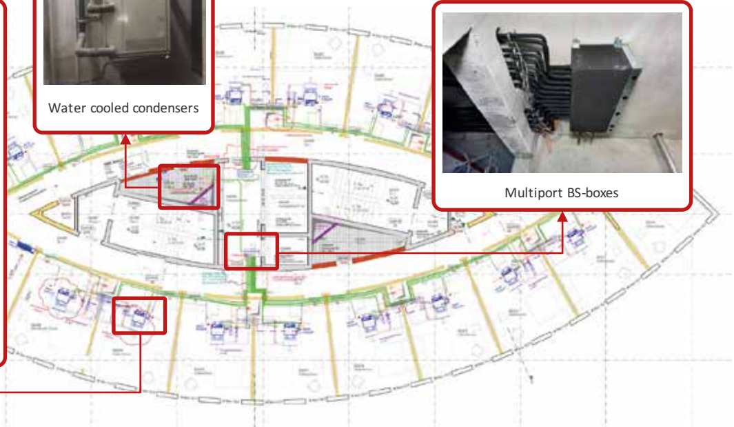
Guestroom installation (low noise slim ducted unit FXDQ)
