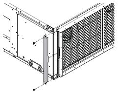
2 Slowly pull out the air filter (composed of 3 equal parts).
