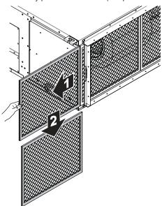
3 Clean the air filter. Use a vacuum cleaner or wash with water. If the air filter is very dirty, use a soft brush and neutral detergent.
