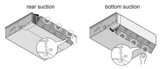
2 Clean the air filter. Use a vacuum cleaner or wash with water. If the air filter is very dirty, use a soft brush and neutral detergent.
