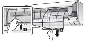
4 Remove the titanium apatite deodorizing filter from the tabs.
