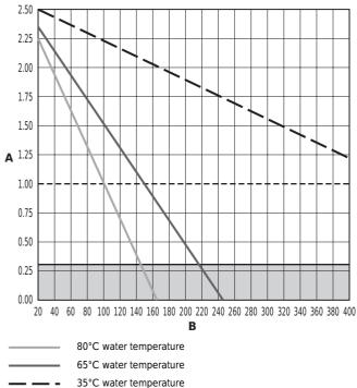
Never change the pre-pressure of the system to a value lower than  $0.3\,\mbox{ bar}$
