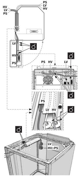
To avoid electric noise problems, be sure that cables are put in the correct bundle as mentioned on the figure.
