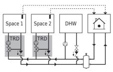
status signal (active/not active) from the corresponding temperature reducing device (TRD)
