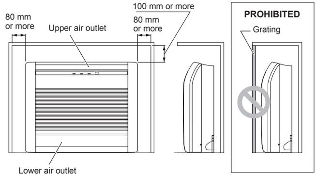
When embedding the indoor unit in a wall, restrict the movement of the horizontal vane for the upper air outlet so that it only operates horizontally. If this setting is not performed, heat will build up in the wall and the room will not be cooled or warmed properly.
