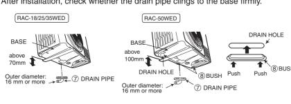
Install the outdoor unit horizontally and make sure that condensate drains away. · In case of using in chilly area
