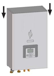
4 Fix the user controller frame to the indoor unit service cover using the screws which had been previously removed during the unpacking procedure.
