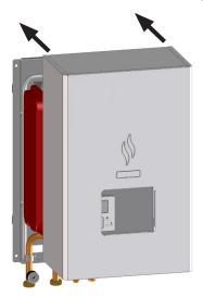
2 Place the holes on the right side of the indoor unit cover over the back plate hooks (x2 locations). When the right side is centred, repeat the operation on the left side. Put the holes on the left side of the indoor unit cover into the back plate frame hooks (x2 locations).
