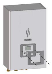
2 Slide the service cover slightly upward and remove it pulling to back.
