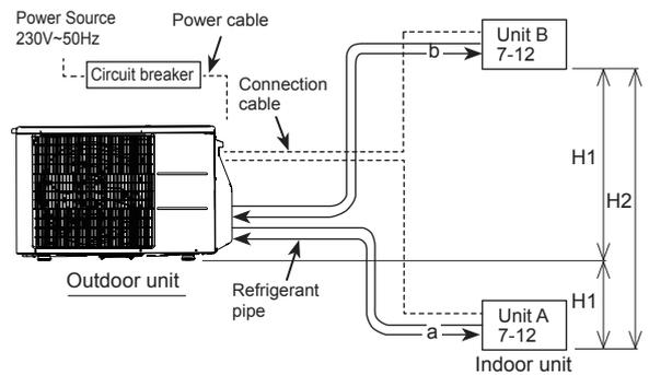
• **Connectable indoor unit capacity type**
