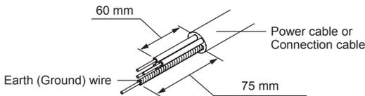
**How to connect wiring to the terminal**
