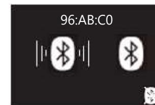
Entering the menu displays whether Bluetooth is currently enabled or not, and shows if a device (App) is currently connected.
