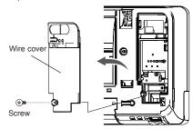
(3) Remove the tapping screw and while minding the cable clamp hook, remove the cable
