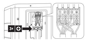
4 Tighten the terminal screws securely. We recommend using a Phillips screwdriver.
