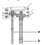
5 Connect the field piping to the accessory pipes using the accessory bend pipes (brazing). Mind the orientation of the bends
