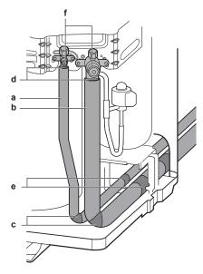
7 If the outdoor unit is installed above the indoor unit, cover the stop valves (f, see above) with sealing material to prevent condensed water on the stop valves from moving to the indoor unit.
