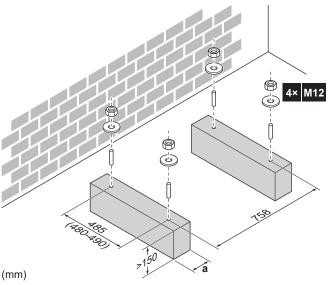
a Make sure not to cover the drain holes of the bottom plate of the unit.
