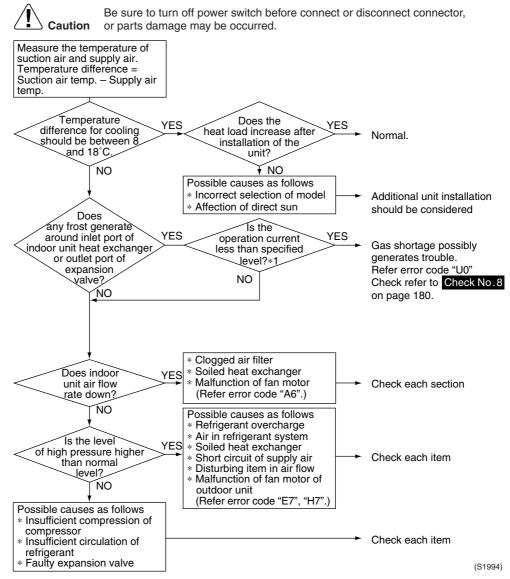
\*1: For operating current, refer to "Electric characteristics" (on page 9) after checking the field system combination (indoor + outdoor).
