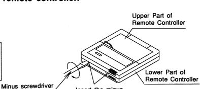
Insert the minus screwdriver and twist lightly to remove.
