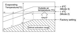
When defrosting conditions are met during heating operation, the indoor unit is demanded defrosting and the following control is performed: **[Defrost control]**
