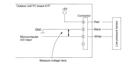
\*2: "Pressure Sensor", pressure/voltage characteristics table.
