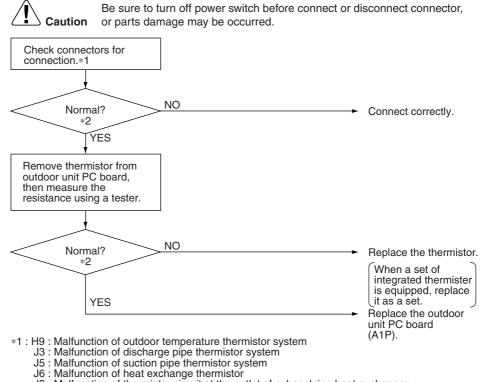
J9 : Malfunction of thermister circuit at the outlet of subcooloing heat exchanger
