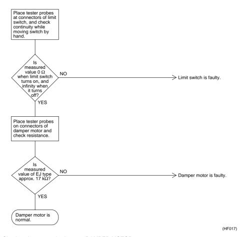
Check resistance and voltage —  $\operatorname{\mathsf{DAMPER}}\nolimits$  MOTOR
