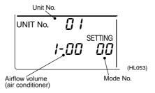
Procedure for entering individual settings (mode No.: 44) The setting is generally the same for all units in the same group control system. However, the setting of selected units can be fixed by the following method.
