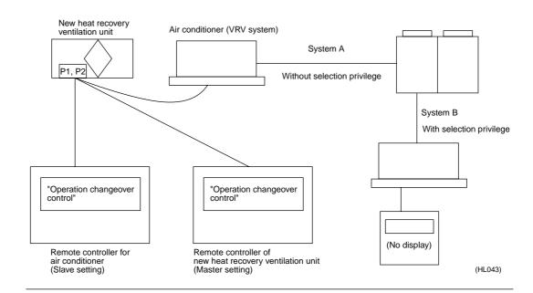
**Display ON/OFF** condition by connection type and cooling/heating selection privilege
