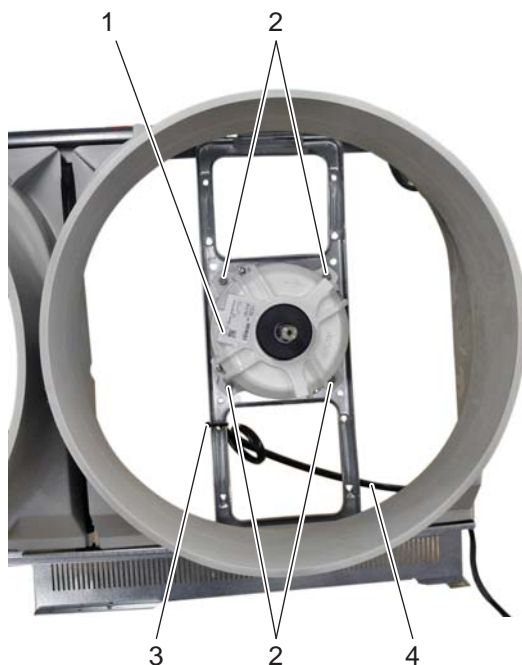
Figure 67 - Removing a fan motor
