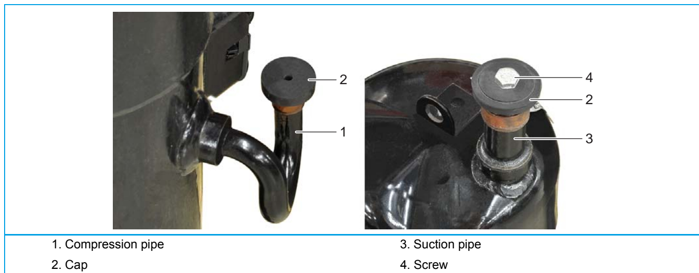
Figure 73 - Installing a new compressor - 1
