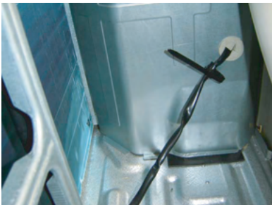
Loose the wire clamp, and remove the lead wires.
