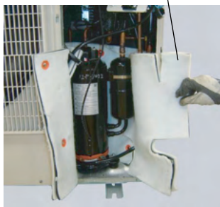
Remove the COMPRESSOR COVER BODY and TOP.
