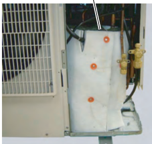
Remove the COMPRESSOR COVER BODY and TOP.
