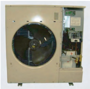
Remove the nut. And remove the PROPELLER FAN. Note at the installation. Insert propeller Fan and Moter shaft reference D cutting position. And the tightening torque at the installation. Tightening torque is from 10 to 12N·m.
