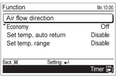
2 "Air flow direction" screen opens. In "Air flow direction" screen, adjustable airflow direction on the relevant indoor unit and its current specified movement are displayed.
