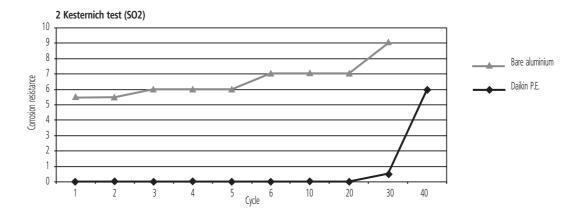
contents of 1 cycle (48 hours): according to DIN50018 (0.21) testing period : 40 cycles
