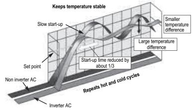
The thermostat can control stable room temperature at ± 0.5°C from set point.
