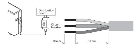
• Use a circuit breaker with a 3 mm clearance of air gap between the contacts.
