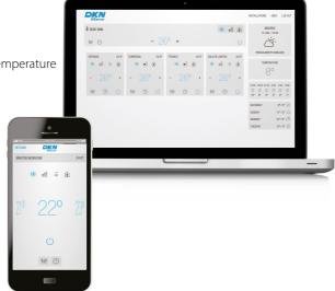
A delay off timer to automatically stop your air conditioning after X hours run can set, as well as multiple time clock schedules. Both of these features can reduce energy wastage.
