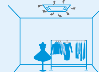
Air distribution with a dusty filter
